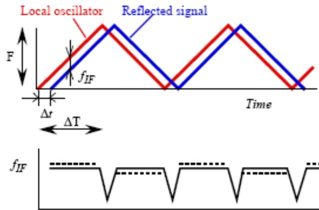
Fig. 1 FM laser radar measurement
