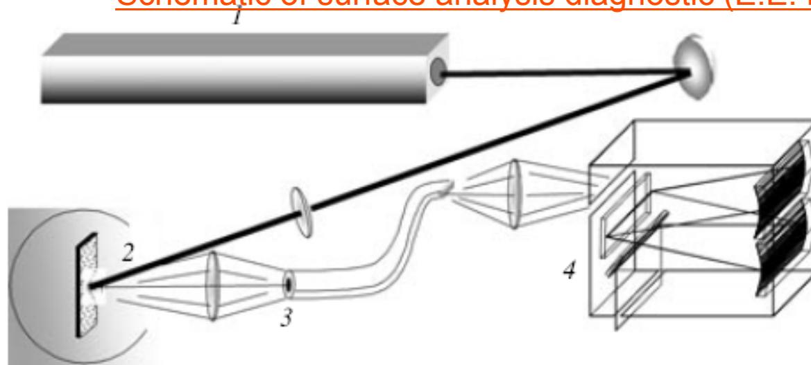
**Fig. 1.** Schematic diagram of the experimental test bench: (1) laser, (2) sample in the vacuum chamber, (3) fiber-optic line, and (4) monochromator with the detection system.
